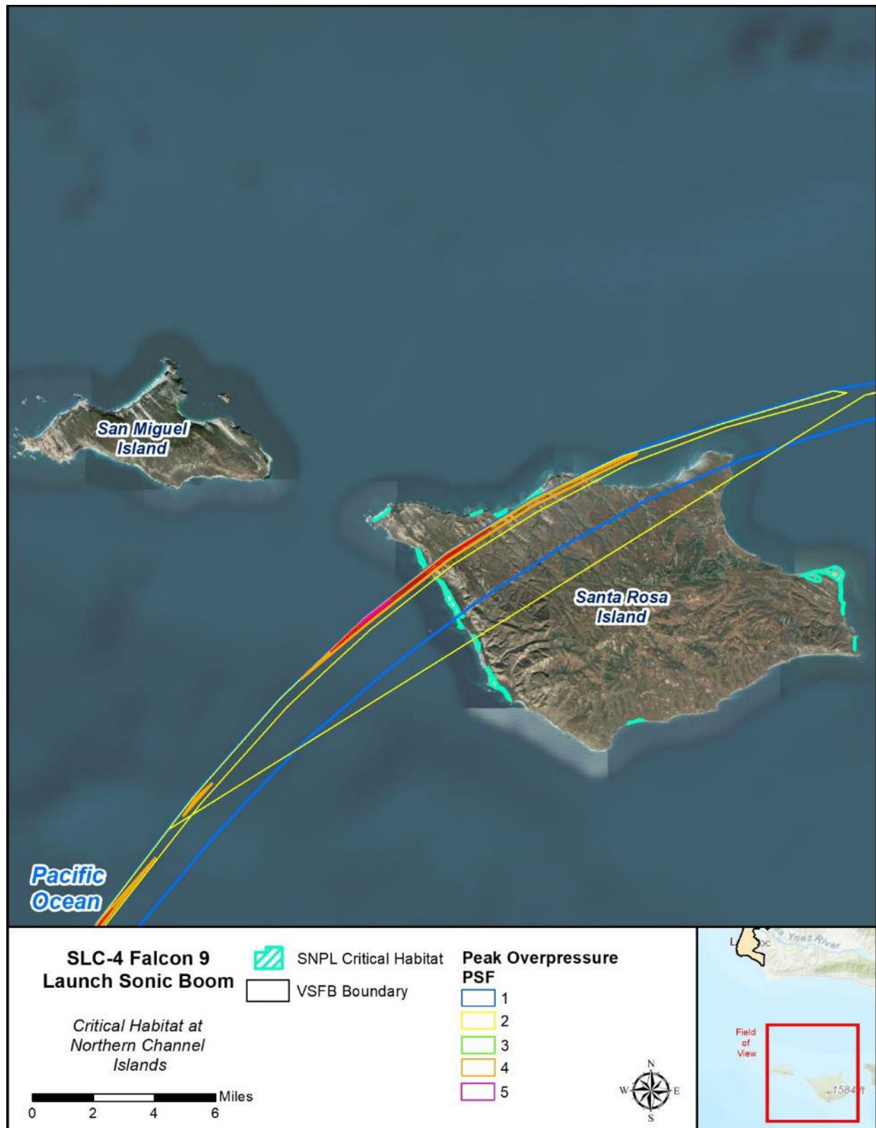
Figure C.0-44. Critical Habitat for the western snowy plover and example SLC-4 Falcon 9 launch sonic boom model results.
