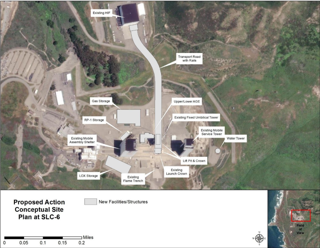
Figure 6A. Proposed Construction Site Plan at SLC-6.
