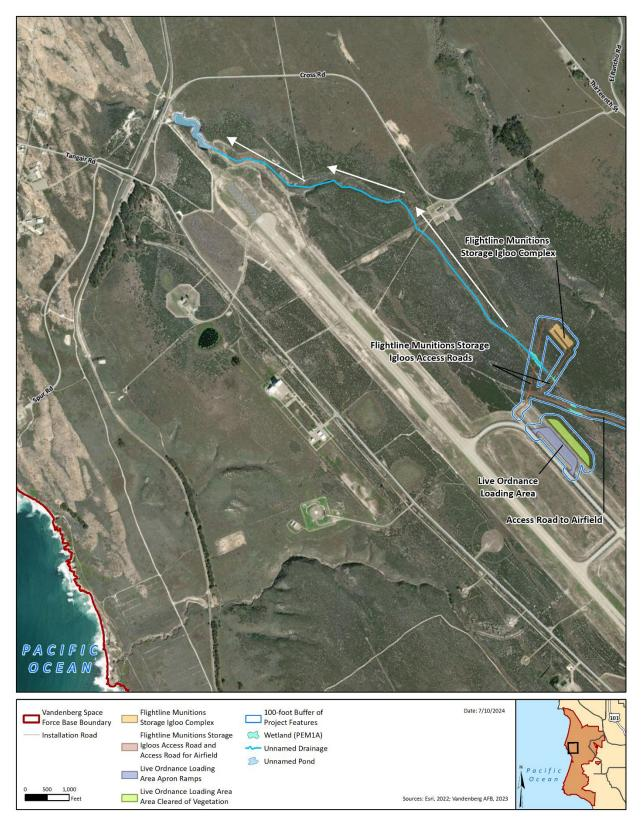
Figure 7. Surface Drainage in the Vicinity of the Flightline Munitions Storage Igloos
