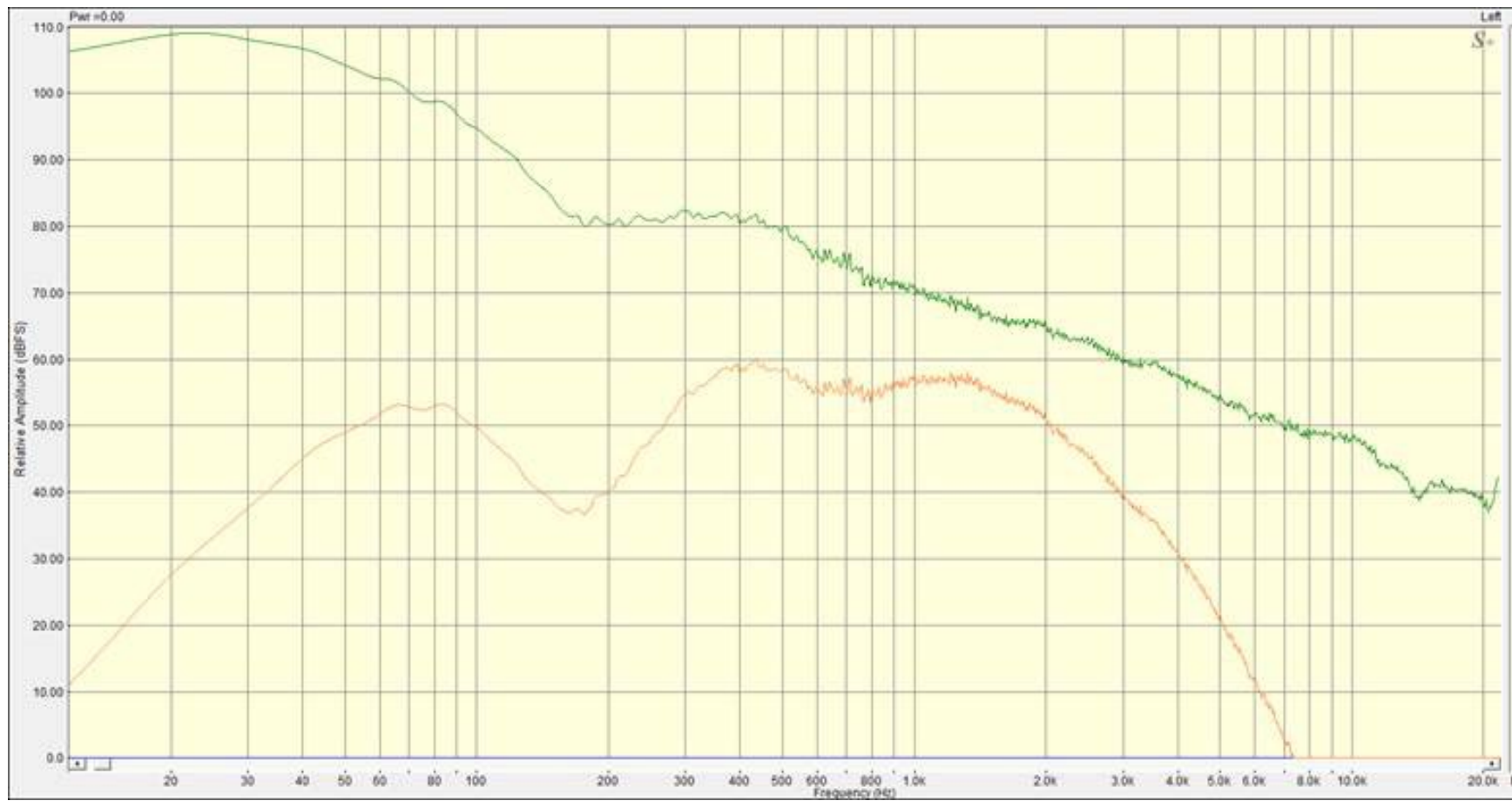
Figure 5.1-16. Launch peak noise level comparison of unweighted (green) versus SNPL-weighted (orange) decibels (note: time waveform recording from the June 2022 Falcon 9 SARah-1 launch).
