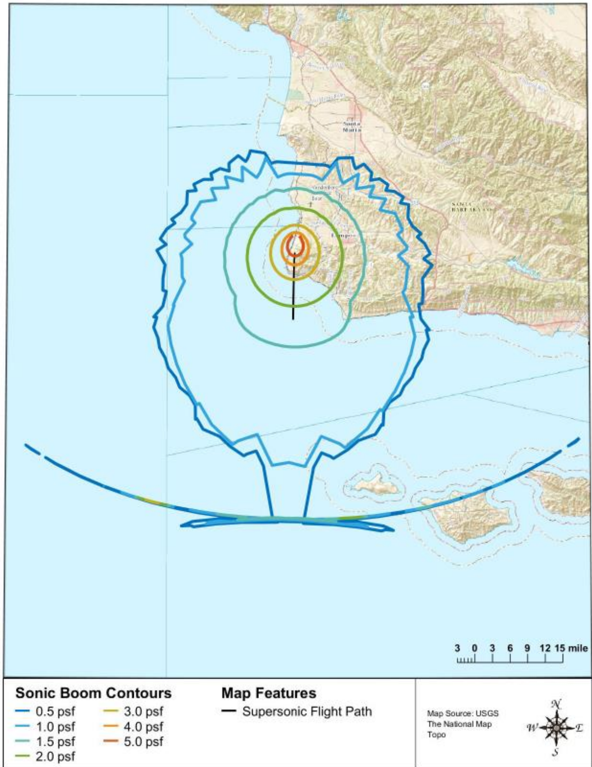
Figure 2-3. Estimated Far-Field Sonic Boom Contours for Falcon 9 First Stage Landing at SLC-4W (Blue Ridge Research Corporation Model)
