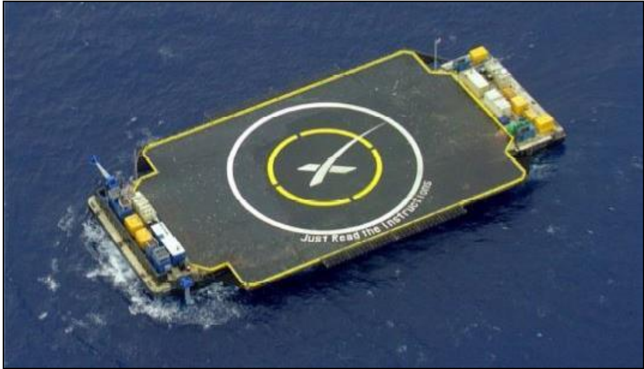
Figure 1-6. Barge Landing Platform
