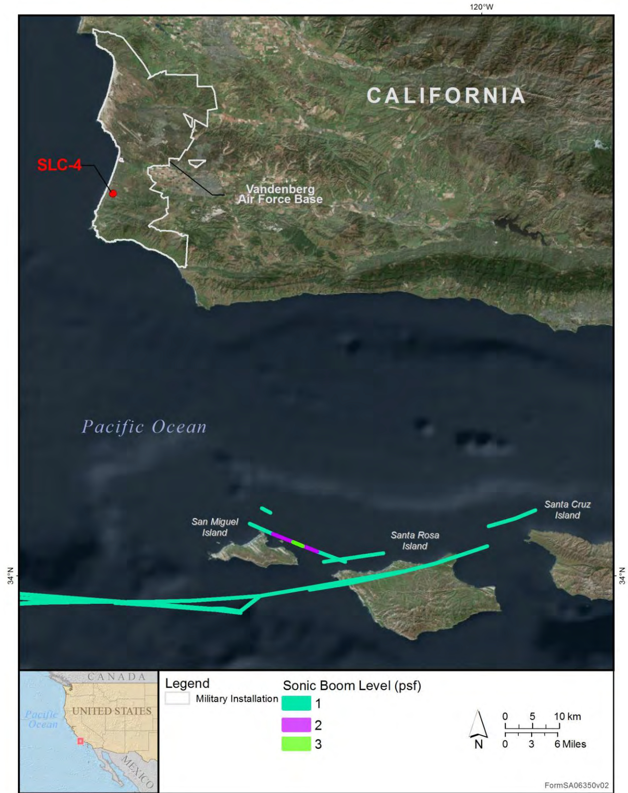
Figure 2-6. Estimated Sonic Boom of Falcon 9 Landing First Stage at the NCI
