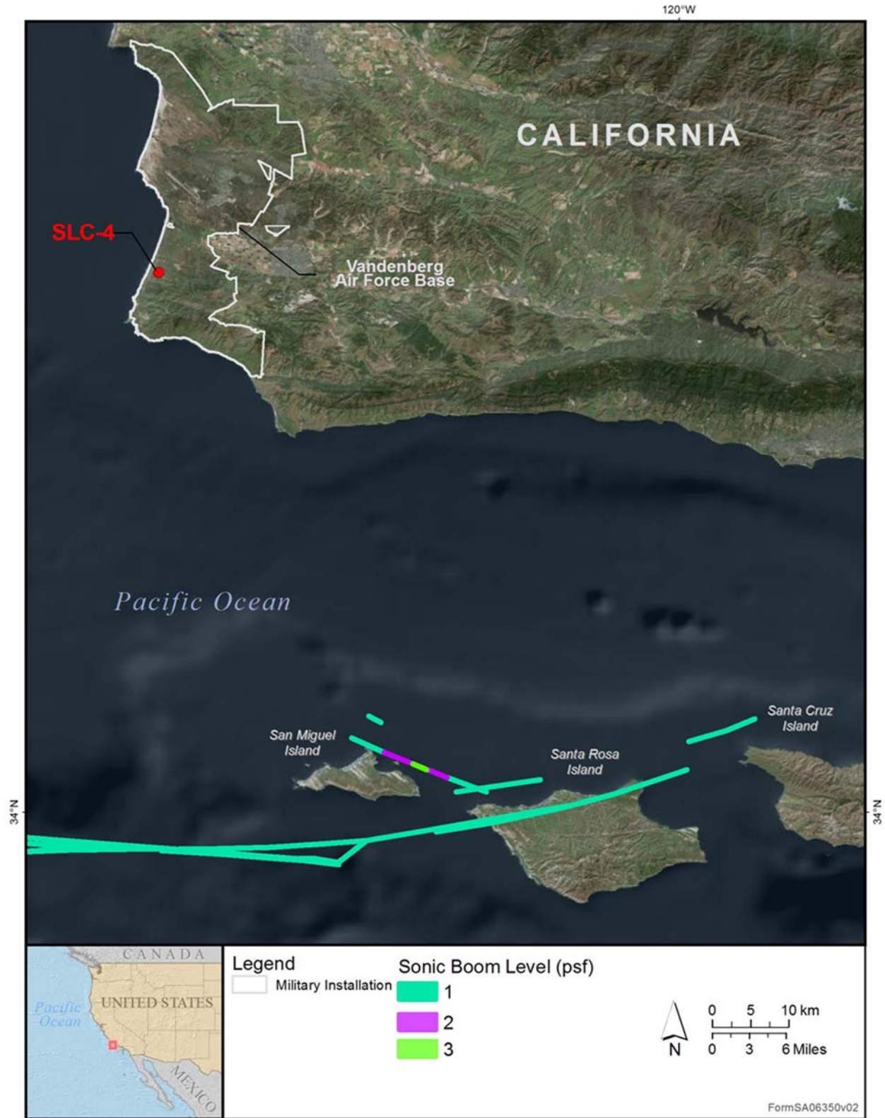
Figure 2-5. Estimated Sonic Boom of Falcon 9 Landing First Stage at the NCI
